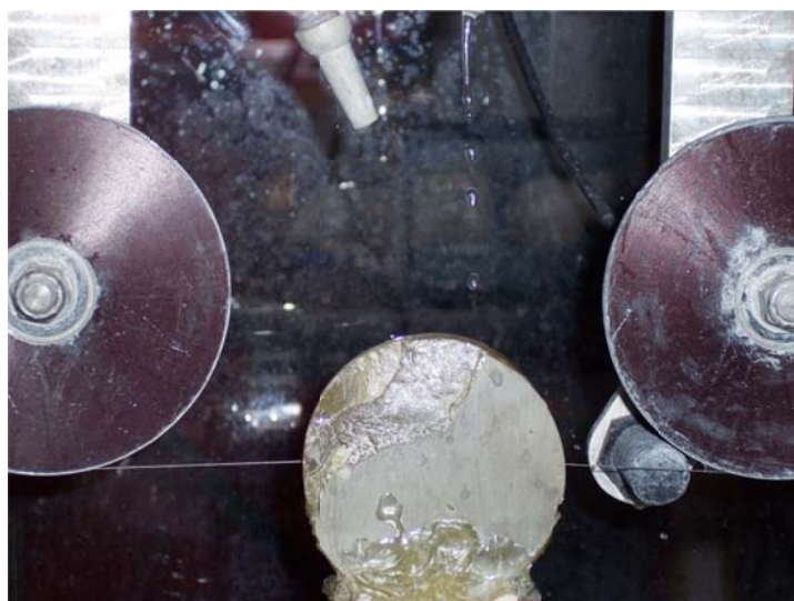
Fig. 2.2 Optical image shows the wire inclination angle with the cutting direction at the entrance and exit from the specimen
